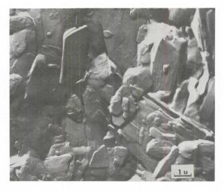
Fig. 7 Electron micrography of lamelar growth of hydrogenated lard
