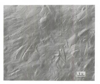
Fig. 8 Electron micrography of needle like crystals of lamellar growth of tallow
