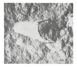
Fig. 3 Electron micrography of hydrogenated oil grain like crystal in hydrogenated soybean oil
