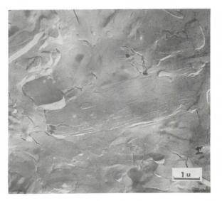
Fig. 5 Electron micrography of large spiral growth of hydrogenated cotton seed oil
