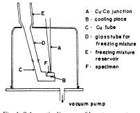
Fig. 1 Schematic diagram of low temperature replica apparatus
