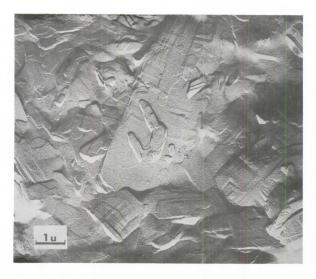
Fig. 4 Electron micrography of spiral growth of hydrogenated palm kernel oil crystal
