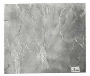
Fig. 6 Electron micrography of crystal flat thin single crystals of lard
