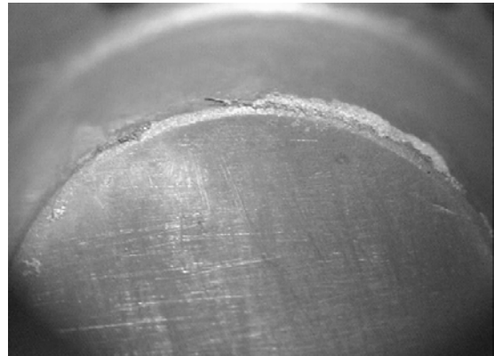
Fig.6.12 Solidification cracking that occurred at the corner.
