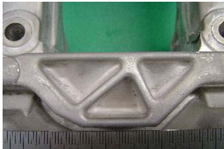
Fig.6.8 Macrophotography at the rib area of the prototype of bearing beam using Al-Ca-Sn magnesium alloy.
