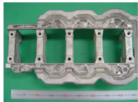
(d) A view from the lower of bearing beam
