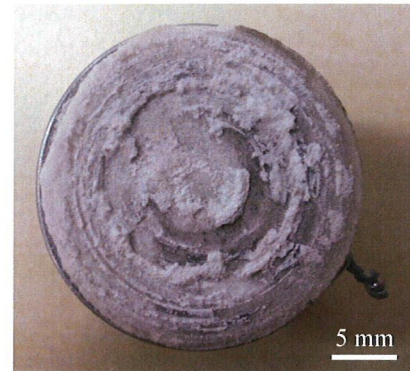
Fig. 5.11. Slip surface of sheared Carrara marble. Experiment are conducted at V=1.3 m/s and normal stress of 3 MPa under H 2 purged atmosphere. Blackish materials stick on the originally white-colored surface.
