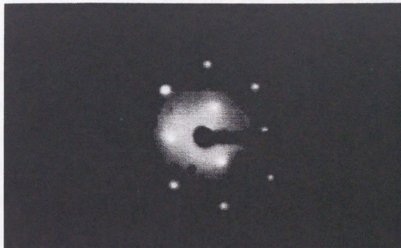
Fig. 4-12. LEED pattern of MnTe epitaxial film grown on GaAs substrate used for the UPS and IPES measurements.
