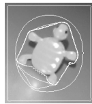
図 19 動的輪郭モデルsnakeの収束過程．最も大きい白線が初期輪郭． Convergence process of snake, the active contour model. The largest while circle is the inisial contor.
