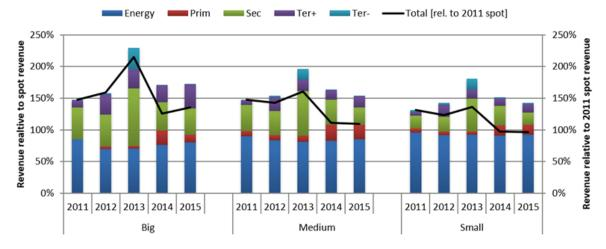
Note: Taken from Schillinger et al. (2017). 'Big' refers to a large scale seasonal storage plant with 100MW, 'Medium' to an in-between sized plant with medium storage volume and 50MW, 'Small' to a run-of-river type plant with limited storage and 22MW. Balancing markets are separated into primary, secondary and tertiary reserves, with the latter being distinguished in positive and negative provision.
