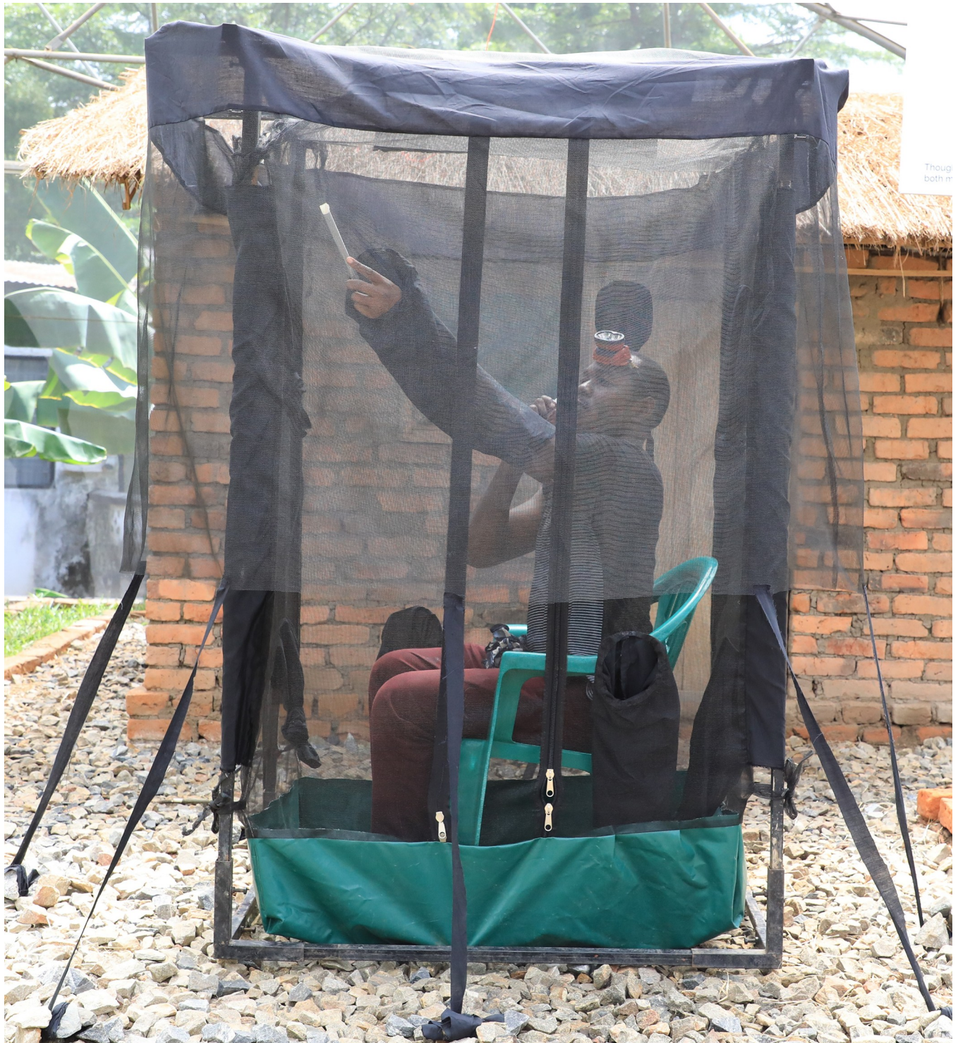
Fig 3. Miniaturized double-net trap (DN-Mini) for comparison of indoor and outdoor mosquito densities.
