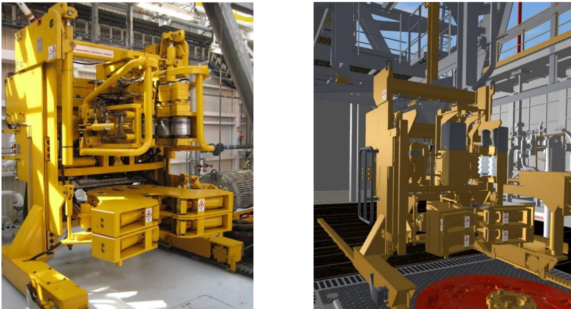
Figure 2-7 HydroTong on an offshore rig and it’s 3D model on the simulator
