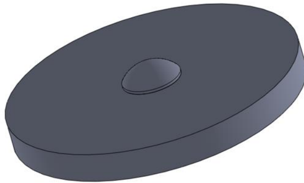
Figure 2.2: Isometric view of the bulged circular sample model
