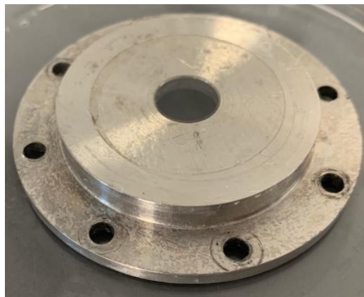
Figure 3.16: PET film attached to the substrate with circular orifice
