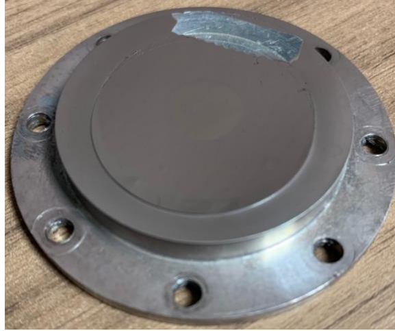
Figure 3.20: Composite (Ge-NW membrane deposited on PET) on the substrate:
