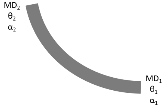
Figure 14: Arbitrary drillstring segment.
