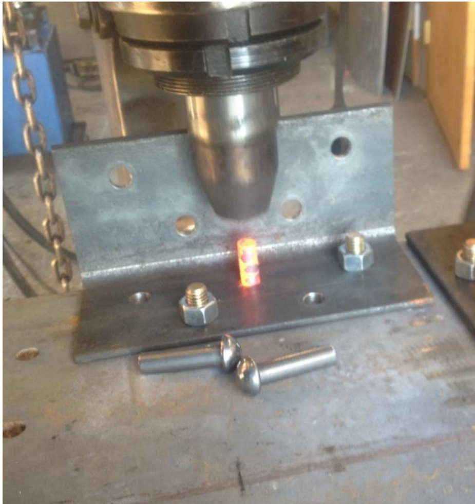
Fig. 3-6: Riveting Process for Laboratory Testing (from Rabalais, 2015)
