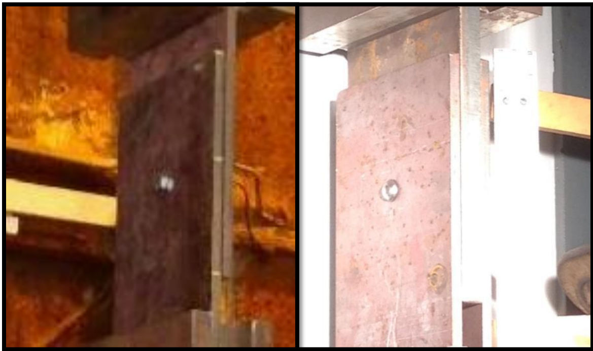
Fig. 3-7: Single Shear with Two 0.5-in. Plates (left) vs. Double Shear with Two 0.5-in. Plates and One 1-in. Plate (modified from Rabalais, 2015)
