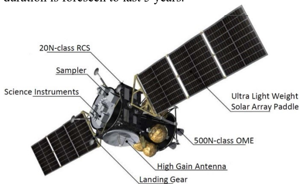
Figure 2. MMX Spacecraft (Credit JAXA)
