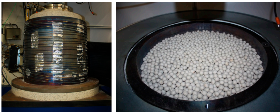
Figure 2. Cylindrical pressure cell with heating wires (left) and filled in particles (right).
