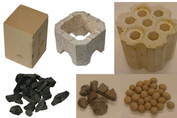
Figure 1. Possible heat storage inventory for a regenerator-type heat storage system.
