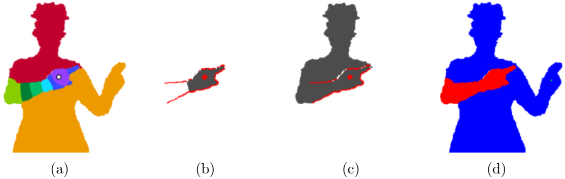
Figure 2.3: Segmenting the arms. (a) Segmented image resulting from clustering probability values of the right arm with mean shift. (b) Potential arm segment (grey) and strong gradient pixels (red). While this binary arm segment B_i does not cut across the gradient, its complement \sim B_i does. This invokes a high cost. (c) Another potential arm segment. The segment B_i cuts across the gradient, also invoking a high cost. (d) Final arm segments (the left segment is minuscule). Only the right arm is valid.
