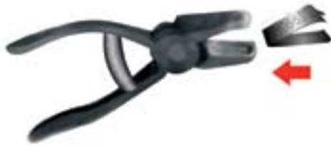
Figure 7 Tag applicator with tag.
