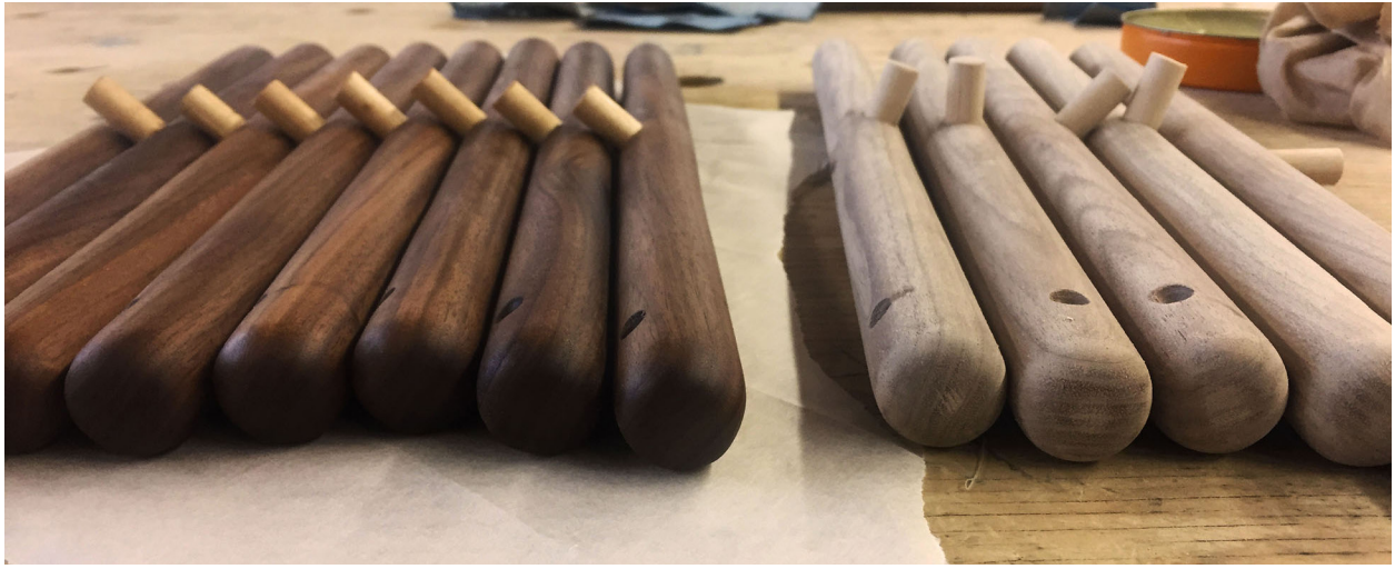
Figure 37: Author, Walnut dowels after and before surface wax , 2019, photograph.
