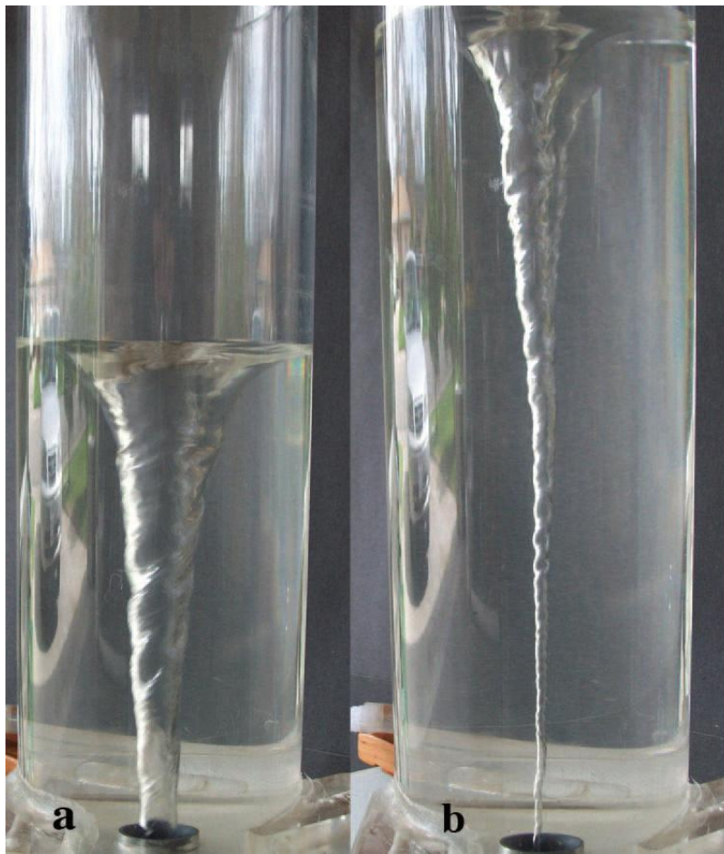
Figure 3.2: Vortex formation above an unrestricted (a) and restricted (b) pipe intake (Shakerin, 2010)
