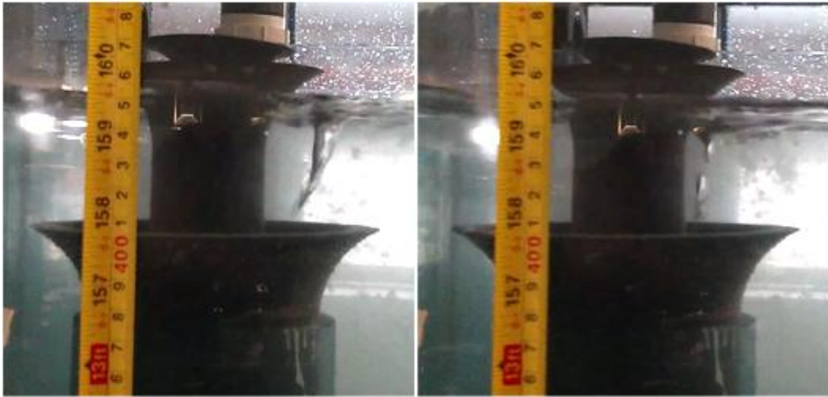
Figure 2.8: An elongated air pocket breaks off an unstable vortex in this snorkel head
