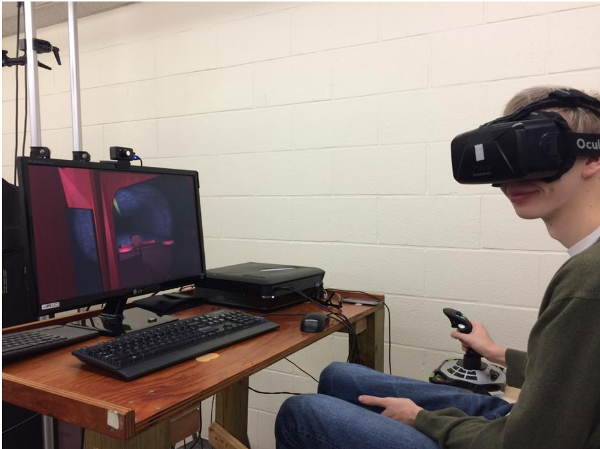
Figure 1. The Situational Awareness Mining Simulator (SAMS) operated on a desktop computer with Oculus Rift headset, joystick and foot pedals. The image on the computer monitor shows what the participant sees in the Oculus Rift headset. The virtual LHD is operated with the driver sitting perpendicular to the direction of travel; therefore, the participant has to turn his or her head to the left to see a forward driving image and to the right to see a backward driving image.
