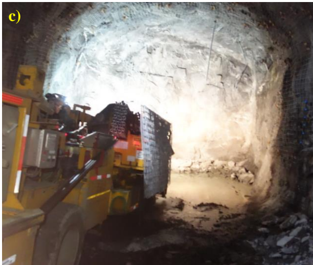
a) Operator gearing MacLean in storage on the 2430 m level b) Bolts, plates and #0 gauge squares on the deck of the bolter c) Traming geared bolter into heading d) Bolts to be installed against front guard rail
