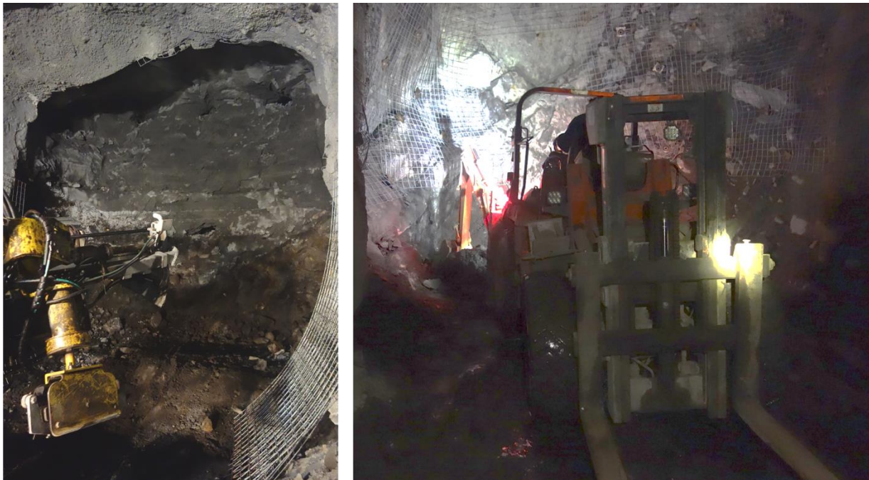
Figure D-3 Left: Overbreak and irregular drift size in sandfill round; Right: Operator removes underbroken sandfill from corners of a drift prior to bolting
