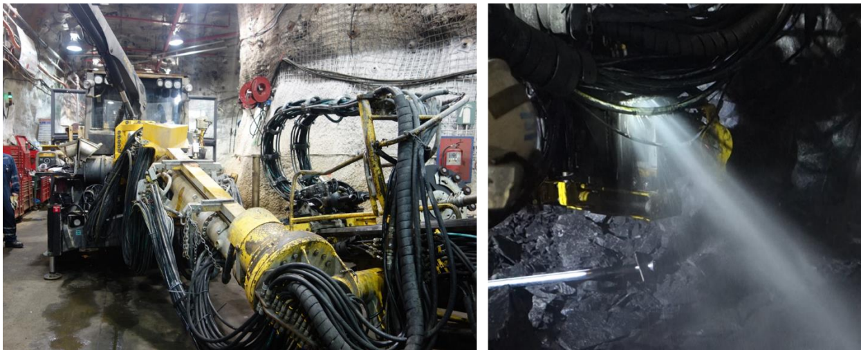
Left: Boltec MC in the Mine C workshop; Right: Hose failure
