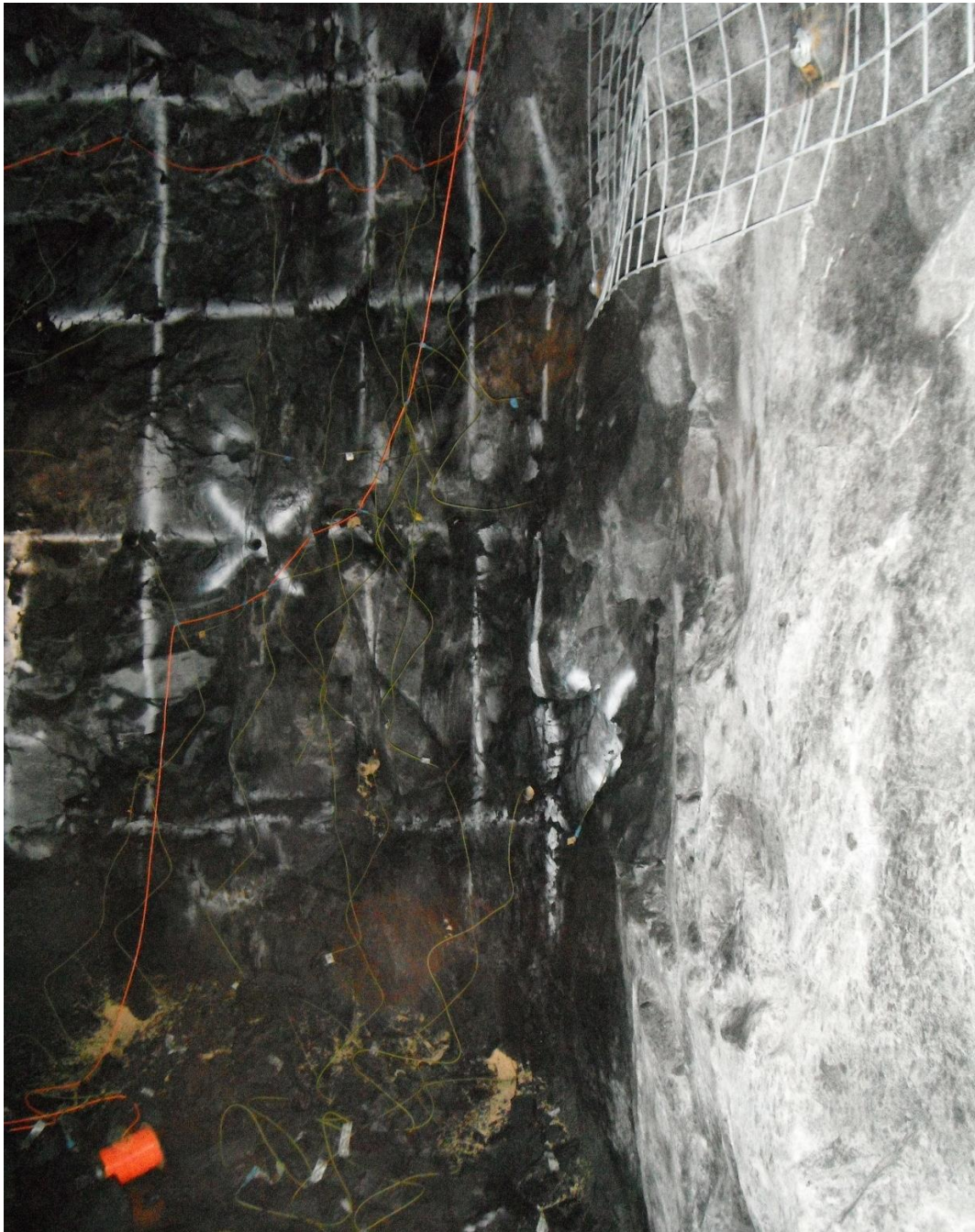
Figure D-1 Typical face loaded with ANFO at Mine A
