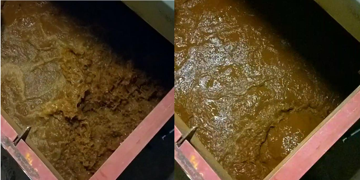
Figure 59: Water surface in the forebay tank during single pump operation at 880rpm (left) and double pump operation (right).
