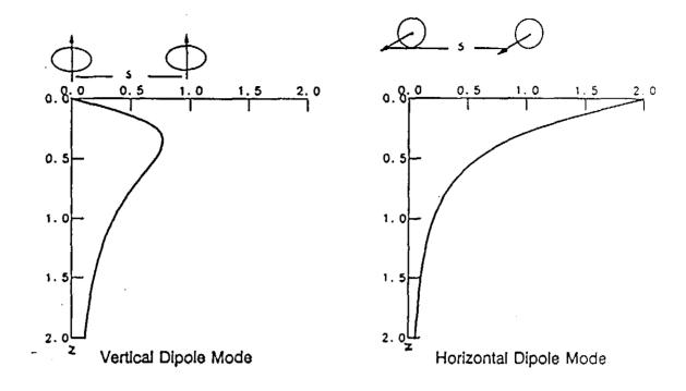
Figure 3.1 Relative responses for vertical and horizontal dipoles.
