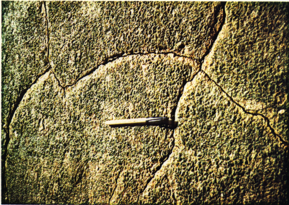
PLATE 12: Moss protonemata on 'pyrrhotite fine' in the Sudbury area. The pH of the surface is 2.5.
