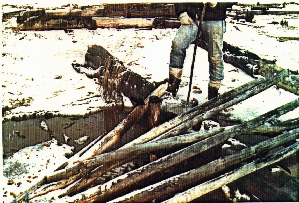
PLATE 7: Drill casing with fresh water flow (sampling site 20).
