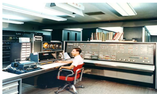
Figure 2.2 1960s UNIVAC computer in operation. Notice the teletype input device to his left. [77]
