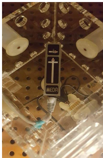
Figure 30. The FVM-400 sensor positioned within the 4D box within the incubator.
