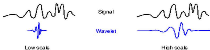
Figure 5-2- Two examples, showing a low-scale and a high-scale wavelet being using to analyze a signal ( http://www.mathworks.com/help/wavelet/gs/continuous-wavelet-transform.html ).
