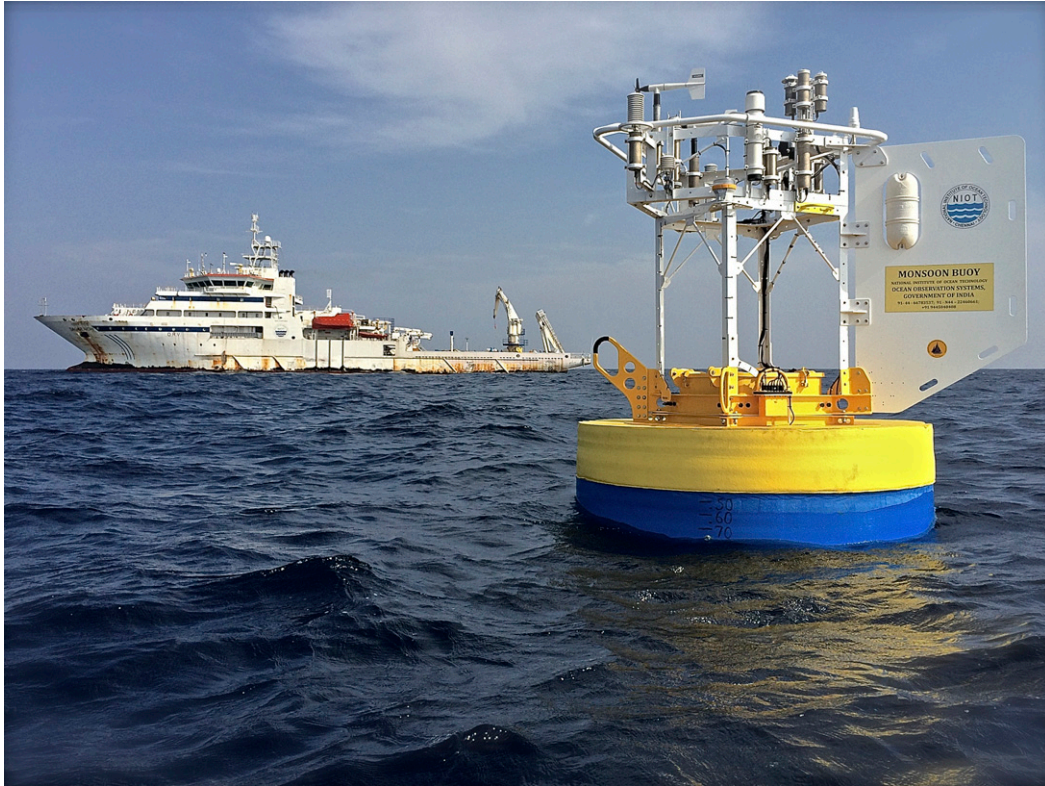
FIG. 2. The surface buoy just after deployment in December 2014, with RV Sagar Nidhi in the background. (Photo by Sean Whelan, WHOI)
