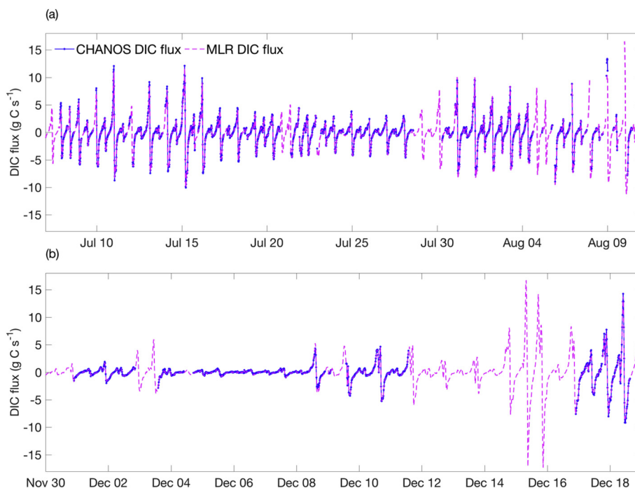
Fig. 3. Time series of DIC fluxes calculated using water fluxes and either CHANOS measured DIC or MLR estimated DIC in (a) July–August and (b) December. Positive values indicate the direction of flux is into the marsh and negative flux values indicate export to the coast.
