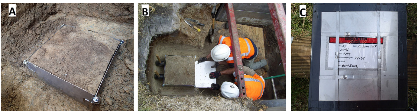
Fig. 3. Depiction of the soil block sampling process: (A) soil is excavated from around the metal box while simultaneously lowering the metal box on the soil horizon(s) to be sampled; (B) once the soil block is full with sample, the bottom plate is pushed into the bottom of the soil block; (C) the top plate is strapped and taped to the side plates and bottom plate (whole box), and the soil block is ready to be shipped.
