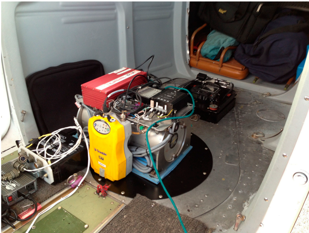
Figure 4. Configuration of the LiDAR scanner (silver), GPS (yellow) and camera (black, background) within the aircraft. LiDAR scanner and camera are pointing through portholes in the belly of the aircraft.
