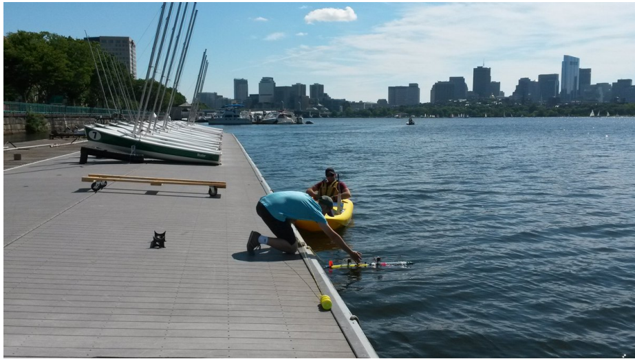
Figure 5-14: UUV was launched from the MIT Sailing Pavilion dock at the Charles River and the array was mounted to the dock.
