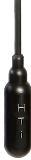
Figure 5-4: Hydrophone element HTI-96-MIN: this hydrophone was used to measure the power spectral density estimate of the micro-UUV. Four of the hydrophones are configured in a tetrahedral array in the nose of the Bluefin Sandshark micro-UUV used in these experiments [6].
