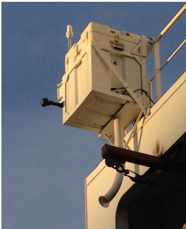
FIG. 2. View of AXIS on the Norröna . The two antennas are for GPS (white) and Iridium (black). The XBT launch chute bends down and away from the back of the ship.
