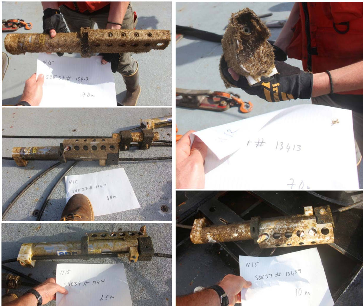
Figure IV-3. NTAS 15 recovered SBE 37 instruments: top left and right (SN 13413, depth 70 m), center left (SN 13411, 40 m), bottom left (SN 13410, 25 m), bottom right (SN 13409, 10 m).
