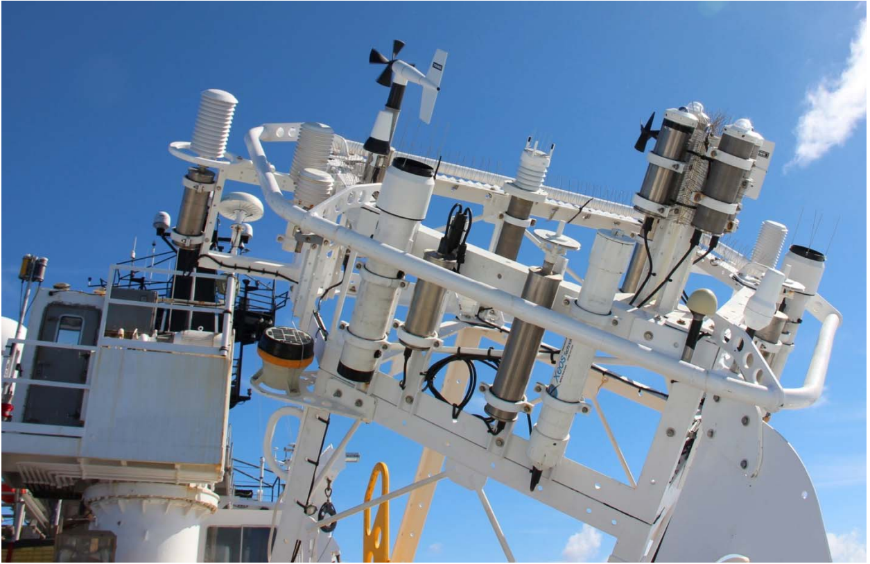
Photo of NTAS-16 tower top prior to deployment, showing bird wire applied to radiometer stalk, PRCs, WXT and inside front rail.
