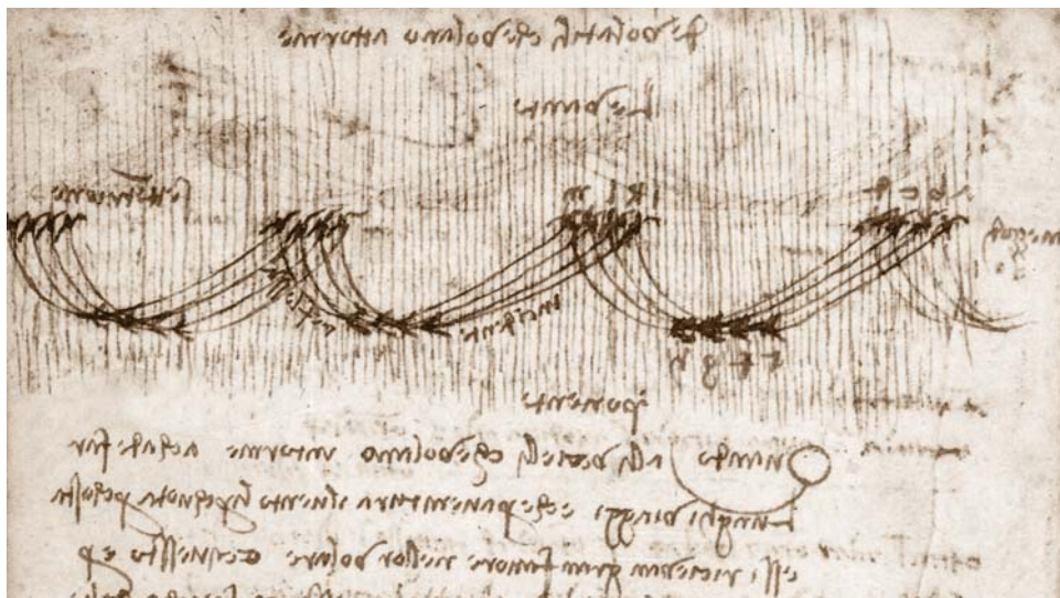
FIGURE 2. ACROSS-WIND dynamic soaring, as illustrated by Leonardo da Vinci in the early 1500s. The nearly straight vertical lines indicate the direction of the horizontal wind, which is blowing from top to bottom in the figure. Reading from right to left, the first phase of the birds' motion involves an ascent that has components out of the plane of the page and against the flow of the wind. The ensuing descent is partially with the wind. The wind direction and the details of the maneuver are described in Leonardo's notes, written in his characteristic reversed, right-to-left style.
