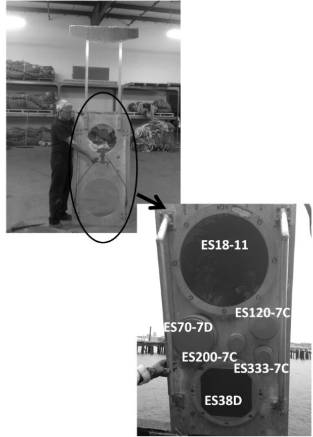
Figure 2. Transducers and aluminum deadweight tow body. Simrad split-beam transducer models are shown for each transducer.
