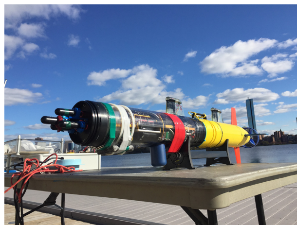
FIG. 1. (Color online) SandShark AUV with acoustics payload and hydrophone array.
