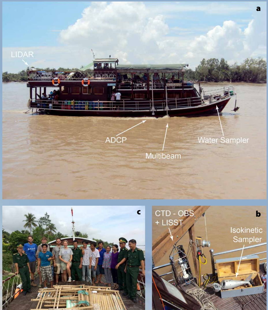
FIGURE B1. (a) M/V Mahogany Star was used to conduct channel studies during the 2014–2015 international study of the Mekong Delta. This image shows the pole-mounted ADCP and multibeam systems. (b) Some of the instruments used to evaluate the mud- and sand-sized sediment fluxes within the tidal river and estuary. The small CTD, the OBS (turbidity sensor), and the laser in situ scatterometry and transmissometry (LISST) profiling system are mounted together in a frame, and the isokinetic sampler is at right. (c) Some of the scientists and crew involved in the 2014–2015 studies are shown here gathered on the upper deck of M/V Mahogany Star .
