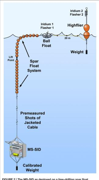
$\label{figure} \mbox{FIGURE 2 | The MS-SID as deployed on a free-drifting spar float} \\ \mbox{system used in this study of ETSP OMZ protist grazing.}$
