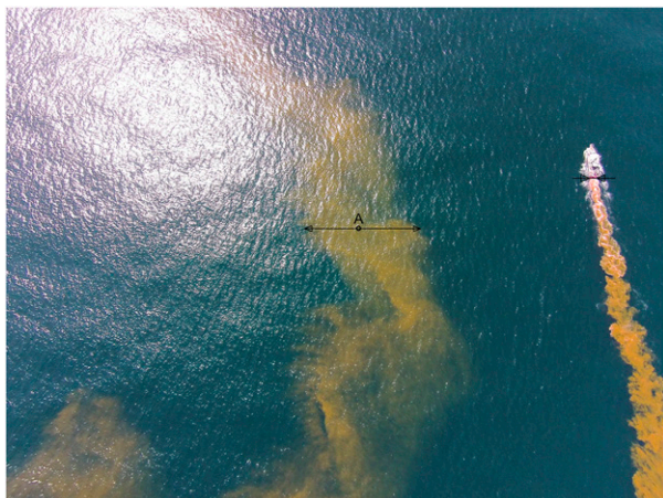
FIG. 3. Georectified aerial image of the dye taken by the quadcopter-mounted camera on 1050 EST 4 August 2014, 23 min after the beginning of the August 2014 dye release experiment. The dye spot in the southwest corner belongs to the initial segment of the spiral release pattern; however, the exact starting point is slightly outside of the image bounds. The R/V Tioga is shown at right; the length and width of the vessel are 18.3 and 5.2 m, respectively. Point A marks the position used to estimate the image-based diffusivity, with arrows indicating the width of the dye streak at point A and behind the ship.
