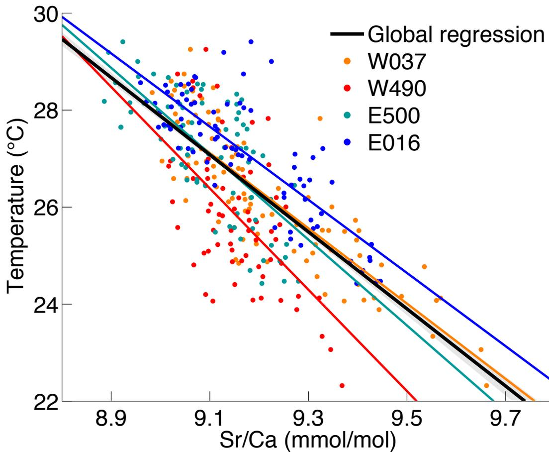
**Figure 2-7:** Global regression of Sr/Ca onto logger temperatures (black, with shading indicating standard error of prediction,  $1.023 \pm 0.003^{\circ}\text{C}$ ,  $1\sigma$ ,  $n = 359$ ). Sr/Ca values and coral-specific regressions for W037, W490, E016, and E500 are plotted in orange, red, blue, and green, respectively.
