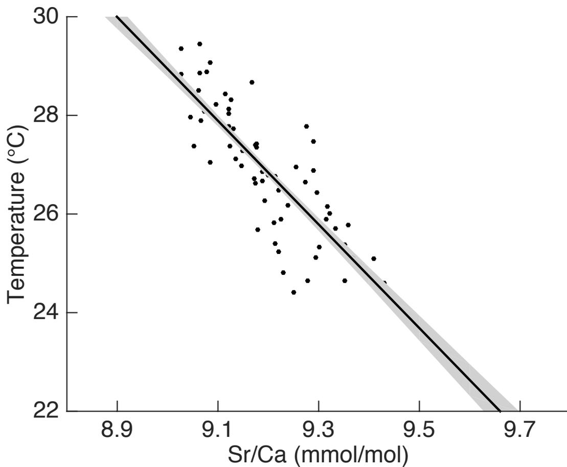
**Figure 2-5:** Regression of stacked Sr/Ca (black circles) onto OISST (black, with shading indicating the error on regression). Standard error of inverse prediction is  $0.779 \pm 0.006^{\circ}\text{C}$  ( $1\sigma$ ,  $n = 65$ ).
