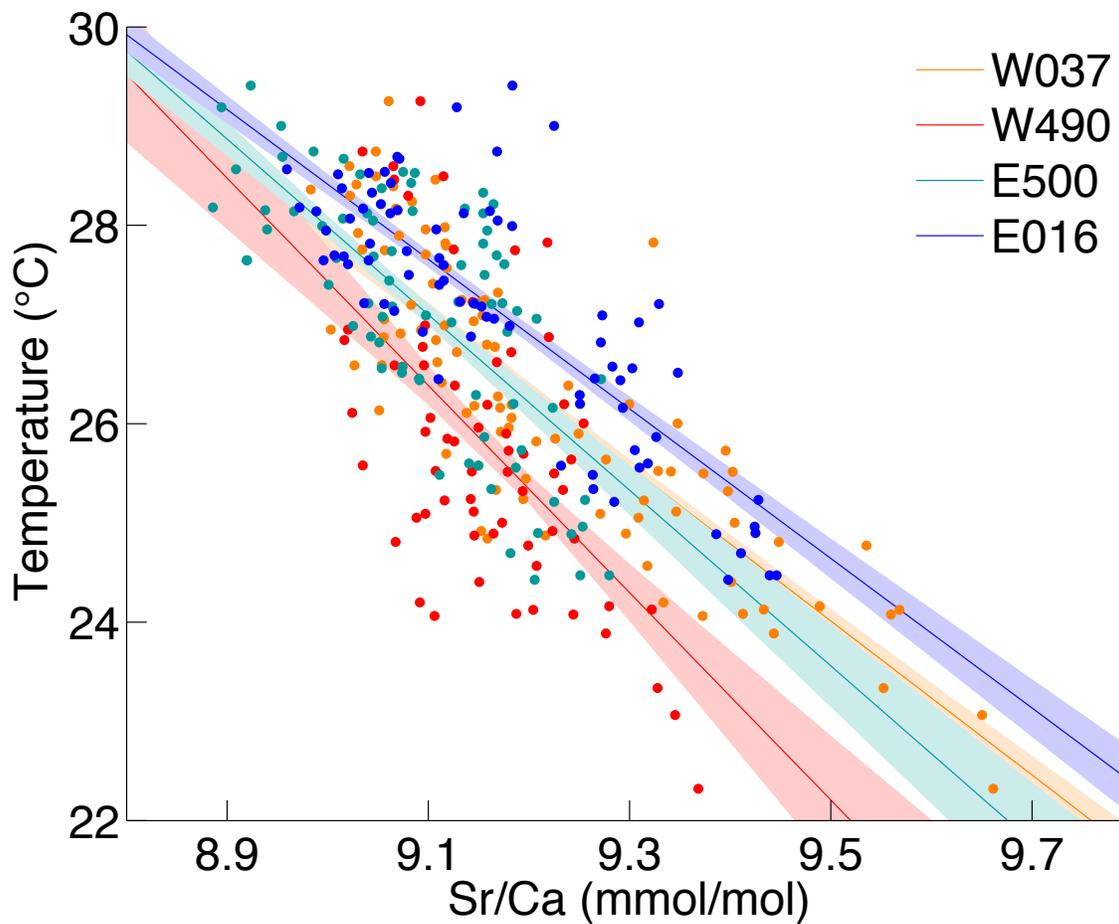
**Figure 2-4:** Regression of *in situ* logger data onto coral Sr/Ca from each of the four cores. Although only the regressions of W037 and E500 are within error, the slopes for all four corals are within error (Table 2-1). Standard errors of inverse prediction range from  $0.744 \pm 0.001^{\circ}\text{C}$  ( $1\sigma$ ,  $n = 78$ ) for E016 to  $1.21 \pm 0.01^{\circ}\text{C}$  ( $1\sigma$ ,  $n = 65$ ) for W490.
