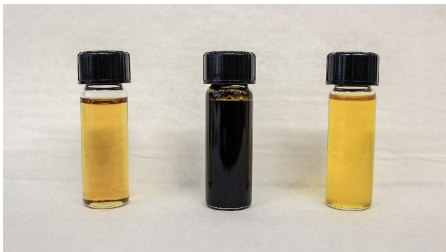
Figure 3. Comparison of Isochrysis and soybean biodiesel fuels. Green Isochrysis biodiesel (middle) is produced by esterification of extracted and purified free fatty acids. Decolorization produces a product (right) with similar properties to commercial biodiesel (left). Please click here to view a larger version of this figure.
