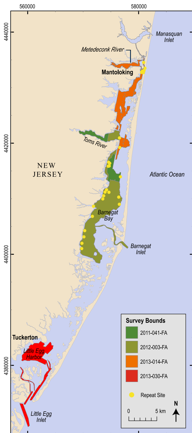
Fig. 3 Map of geophysical survey coverage collected over 2 years; areas in green were surveyed prior to Sandy, and areas in red and orange were surveyed after the storm; yellow circles indicate locations of 26 sediment sampling sites visited before and after the storm
