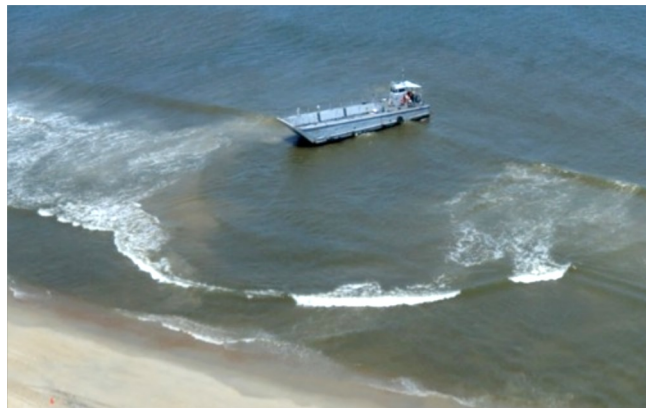
Figure 1.3. Photograph of a landing craft that was used to dredge shore-perpendicular channels across the surf zone by suspending sediment with its propellers near Duck, NC in 2012.
