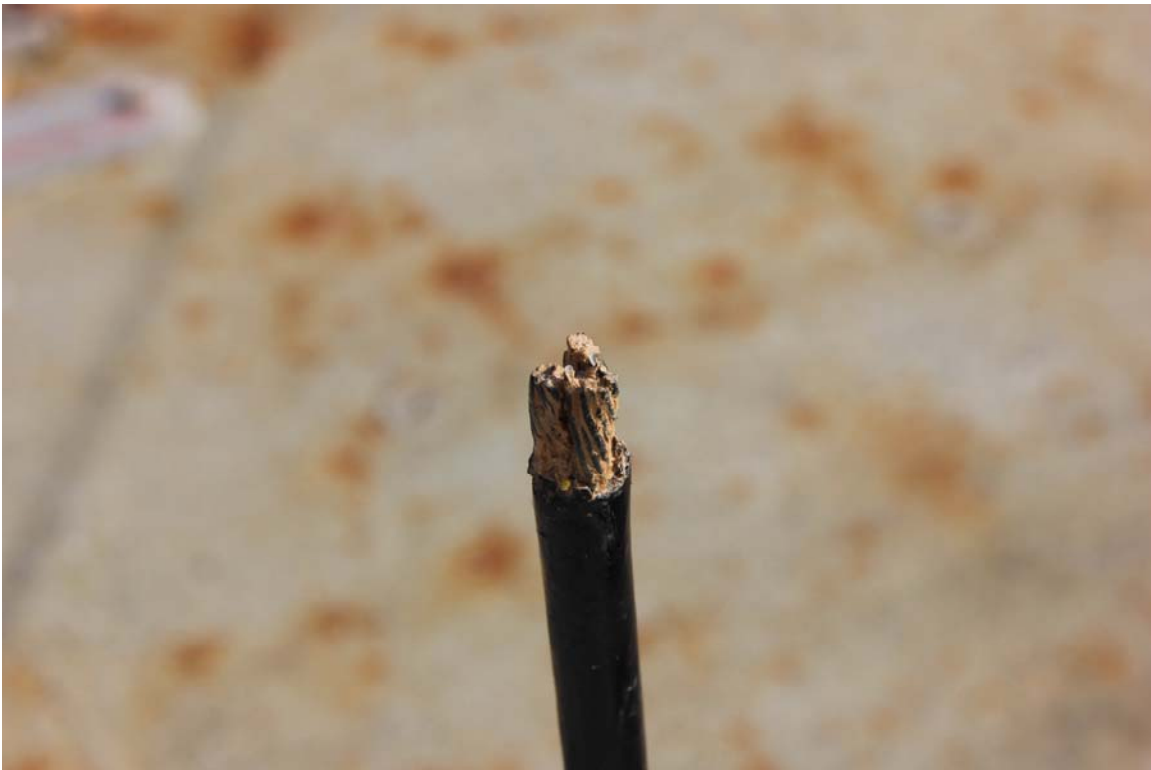
Figure 4-1. Breakup of NTAS-13 mooring, as recovered on December 15 2014.
