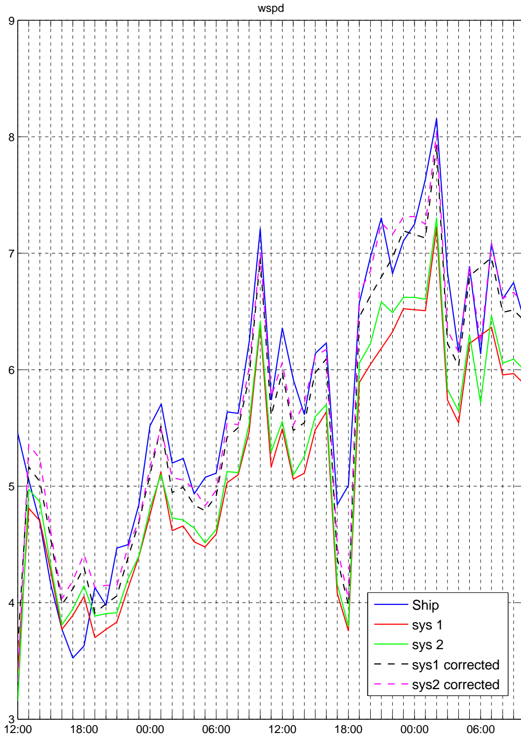
Figure 3-14. Same as Fig. 3.7 but for wind speed (WSPD, \text{m s}^{-1} ). Dashed lines are buoy ASIMET adjusted to height of ship's sensor.
