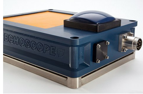
(b) Coda's Echoscope 3D Sonar Scanner [21].
