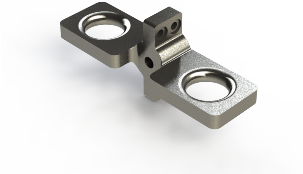
Figure 3-7: The anchor is comprised of two separate and symmetrical pieces that attach around the base of the tap portion of the piece. There is enough clearance between the anchor and the tap sleeve to allow for its independent rotation from the rest of the mechanism. In the situation where the lifting lines are attached to the mechanism equipped onto vehicle before deployment, the insertion of the tap sleeve without the anchor's free rotation would result in the entanglement of the lines.
