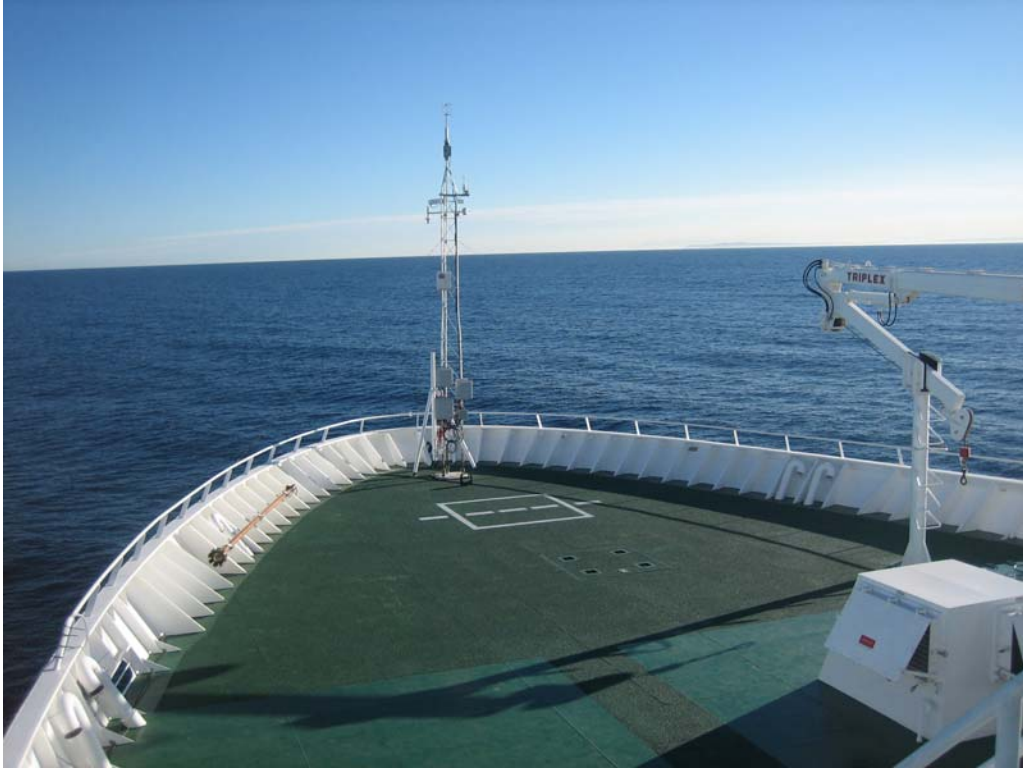
Figure 3-12. ESRL meteorological tower on bow, O2 deck.
