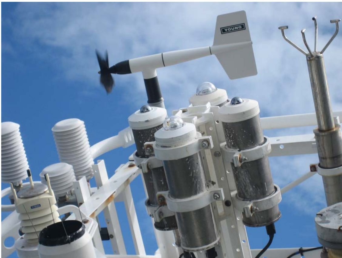
Figure 4-24. Picture of Stratus 13 buoy after recovery (IMG_1484.JPG). Note drooping on aft SWR.
