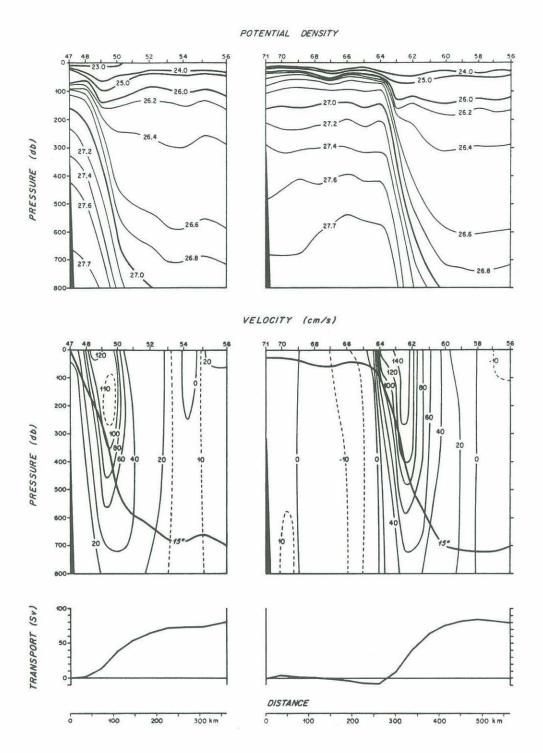
Figure 3: Density (upper panel), velocity (cm/s, middle) and integrated transport (Sv) for the "real" salinity data on the EN88 transects of the Gulf Stream.
