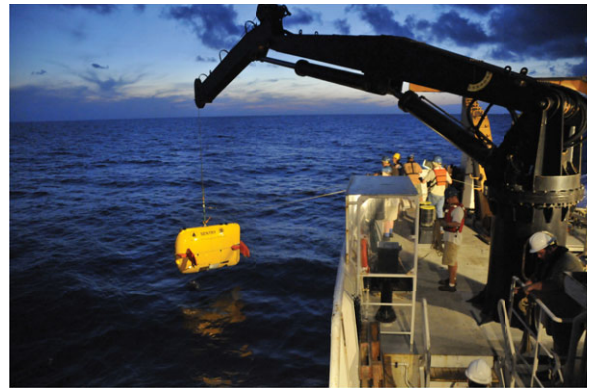
Figure 14. The National Deep Submergence Facility (NDSF) AUV Sentry is an unmanned oceanographic research vehicle that dives as deep as 6,000 m to perform various scientific missions. Sentry navigates primarily by DR with a FOG and DVL. The FOG is located in the main pressure housing, roughly amidship and just below the name label. The DVL is on the keel just aft from the bow. The large separation between these sensors on a vehicle that may deform under extreme pressure (even slightly) motivates our study of stable, in situ sensor alignment methods (photo credit: D Yoerger, ABE/ Sentry Group, WHOI).
