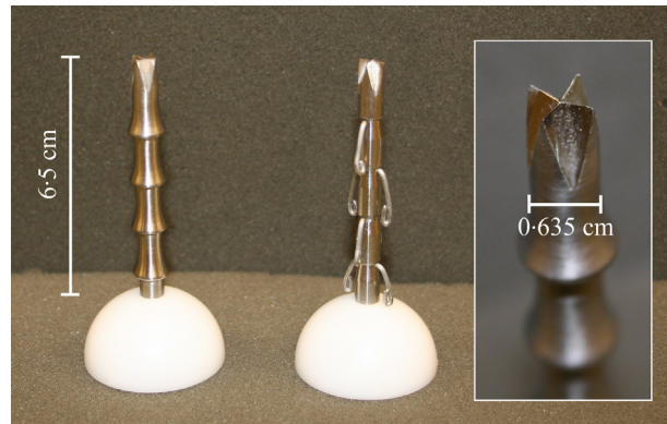
Fig. 1. Needles used in humpback whale field trials. Needle at left features four tapered cupped rings rising 0.16 cm above the needle shaft, while the needle at right features four curved 316 stainless steel pins. Each needle is attached to a white hemispherical delrin 'stop'. Inset shows cross design of needle tip with four cutting blades and side vents.
