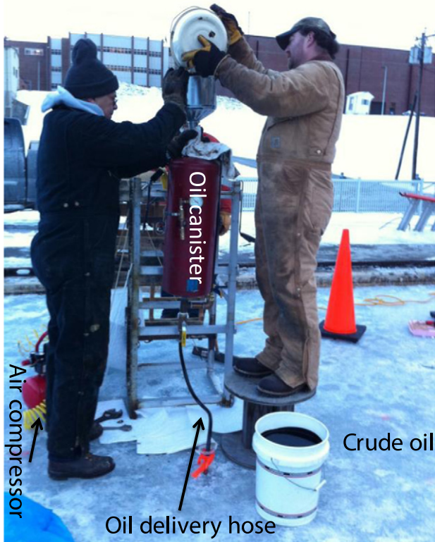
Fig. 2. Photograph showing the filling of the pressurised oil delivery system. This system allowed oil to be deployed efficiently and effectively as well as constraining the oil to the experimental hollow under the sea ice. No evidence of oil spreading beyond the hollow was seen.
