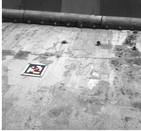
Figure 4-9: An AprilTag captured by the periscope camera on the hull of the Saratoga , Newport, RI. This is a cropped detail of the upper left quadrant of the camera frame.
